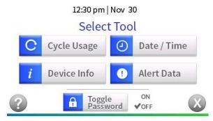
The Cycle Use Information History screen can be reached by selecting the "Cycle Usage" button. It will display the past cycles run on the unit which may be scrolled through using the arrows on the right of the screen. Additionally, there will be a "Back" button to return you to the Select Tool screen and a "Delete?" button. The "Delete?" button will prompt an alert to confirm the previous cycle's information is deleted.
