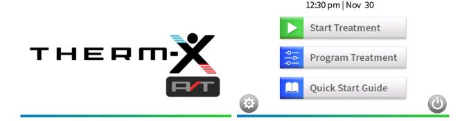
If you have already programmed the therapy treatment, follow all instructions in the 'Preparing the Therm-X for Use', including unpacking the machine, filling the coolant tank, and attaching the hose and garment. Then select the "Start Treatment" button from the Home screen.
