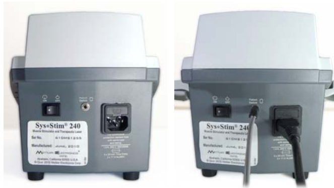
Figure 3.3— Sys*Stim 240, Back View Showing the On/Off Switch and Power Cord and Patient Safety Cable Connections
