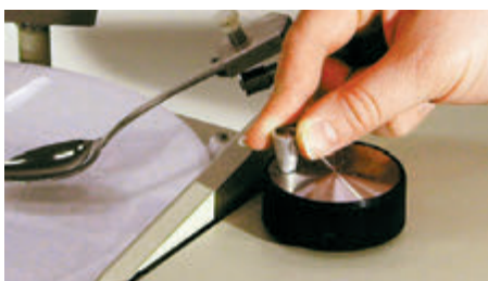
Turn the large black knob to set the height of the feeder.
