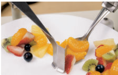
The Pusher moves the food onto the spoon once the switch is released.
